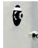
USCITA FOG / FOG OUTLET: raccordo push-in FOG 5mm per tubo polyamide 5mm push-in fitting for polyamide tubing (1/4" or 3/8" su richiesta / upon request)
